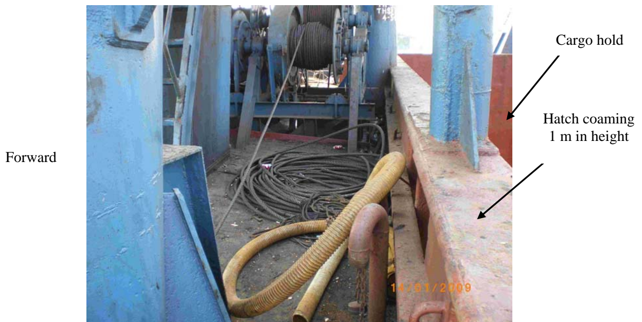
Fig. 7: Main deck at the port forward part of “Pak Lee”
