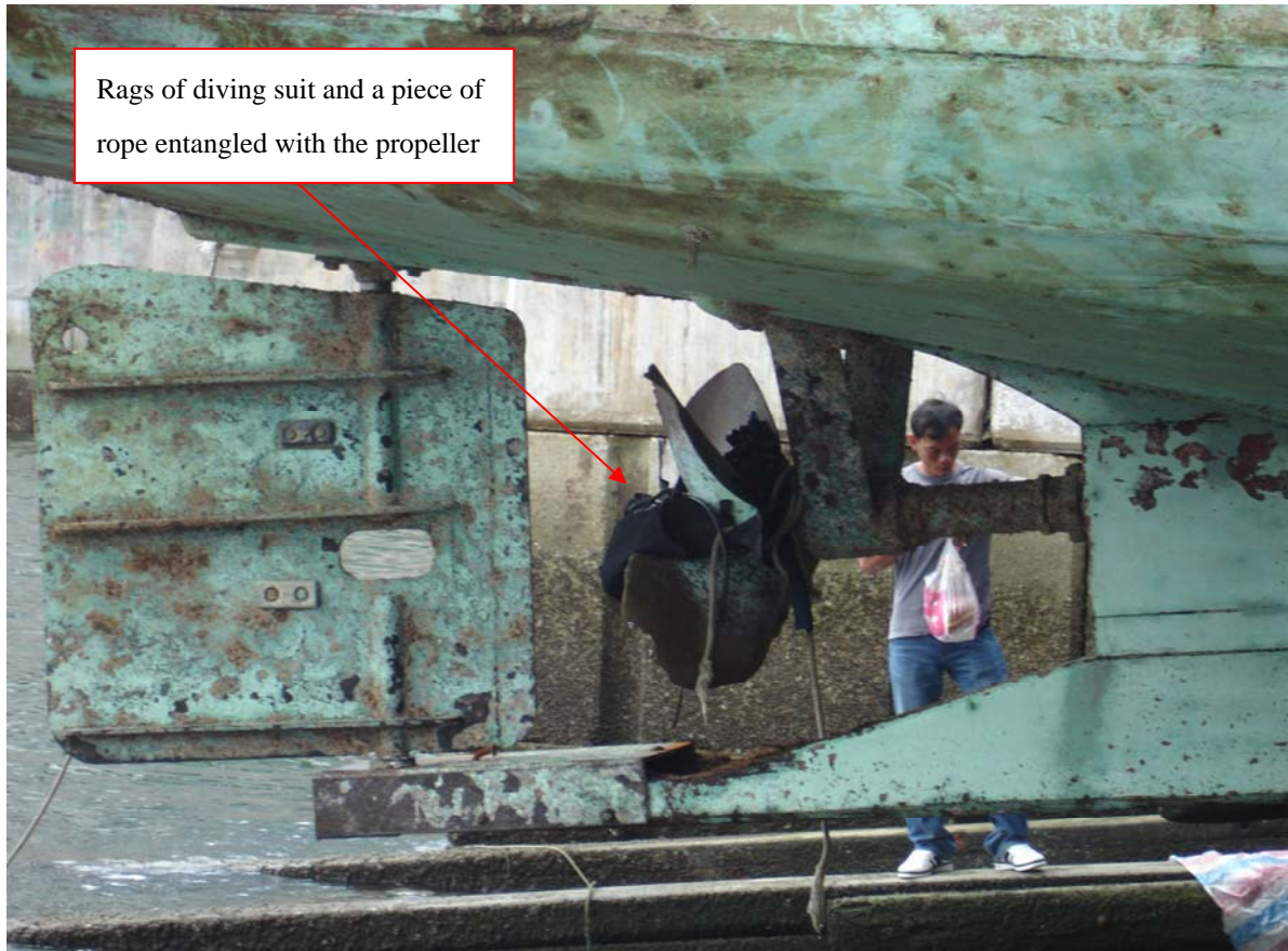
Figure 4 – Diagram showing the propeller of Crescent Island
