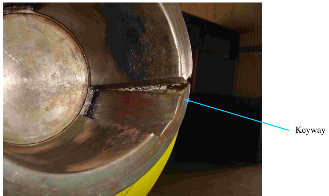
Fig.22: Inside View of the Deformed Upper Coupling
