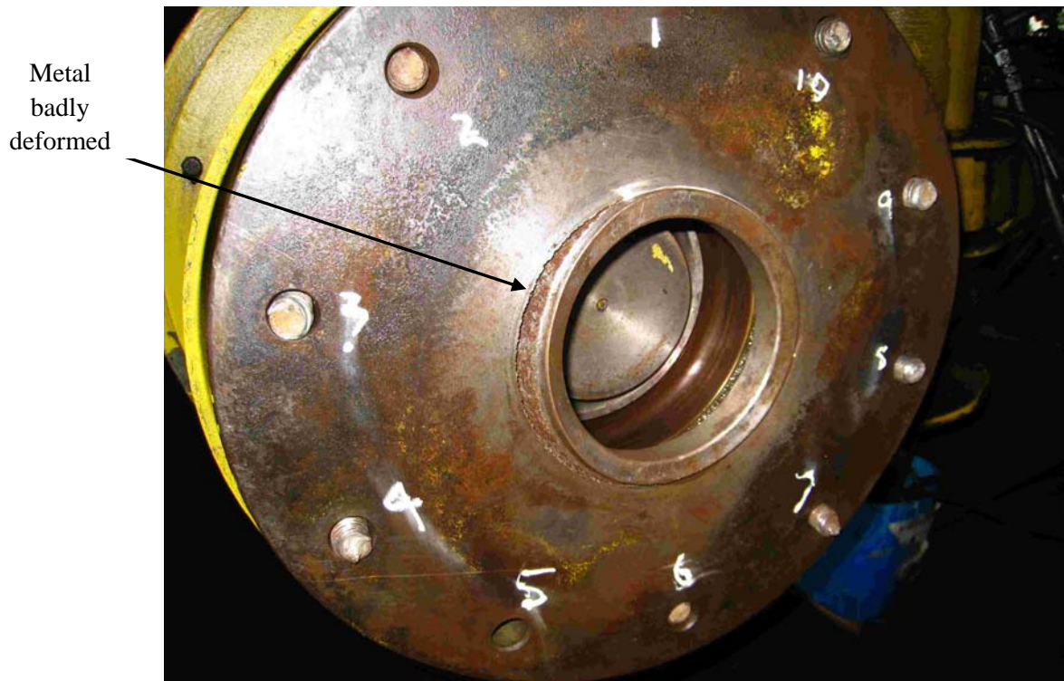
Fig.16: The Bottom Side of the Deformed Flange of Lower Support Bush
