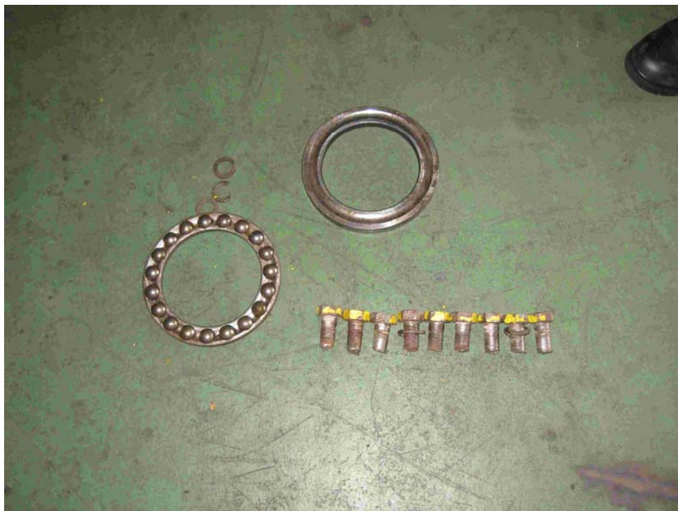
Fig.17: Nine Broken M20 Bolts of the Lower Support Bush and Parts of Thrust Bearing
