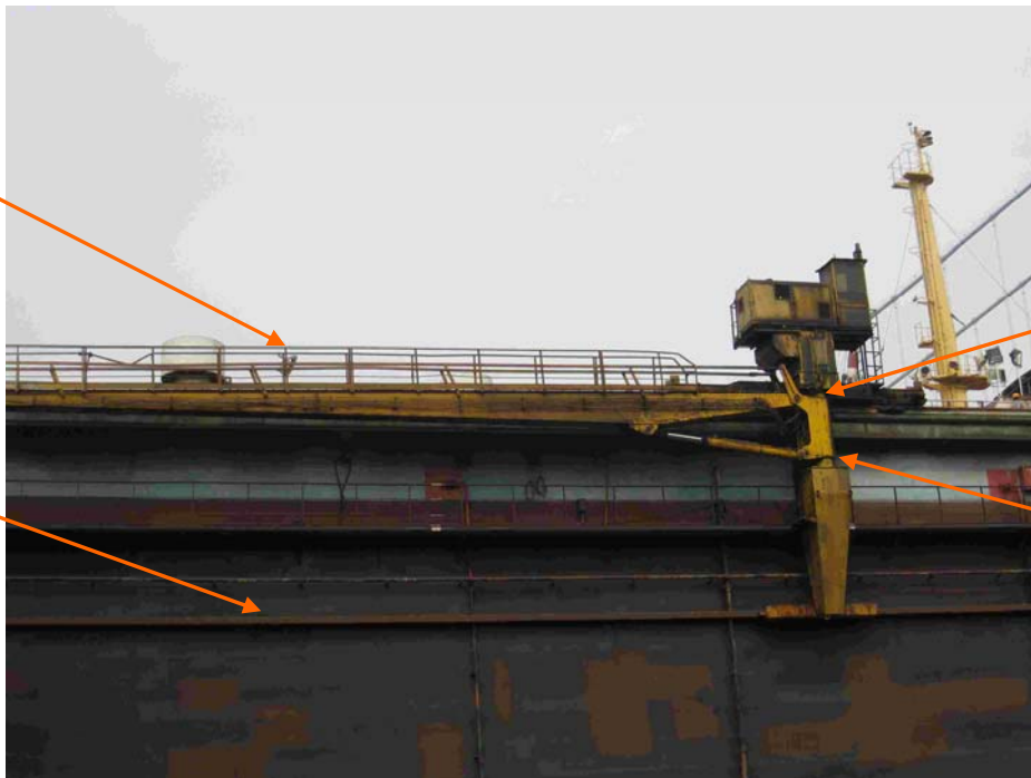
Fig. 19: The No.3 Dock Arm on board Floating Dock "United"
