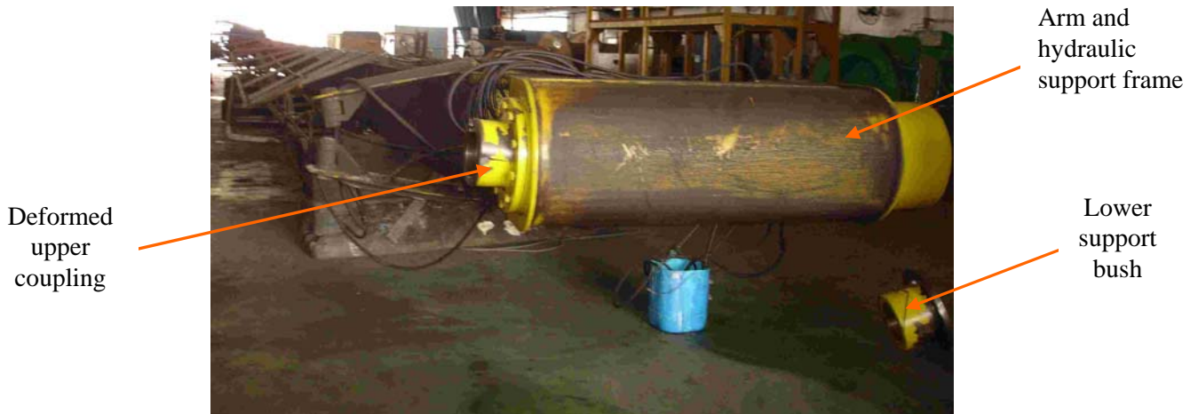
Fig.12: The Arm and Hydraulic Support Frame of No.2 Dock Arm
