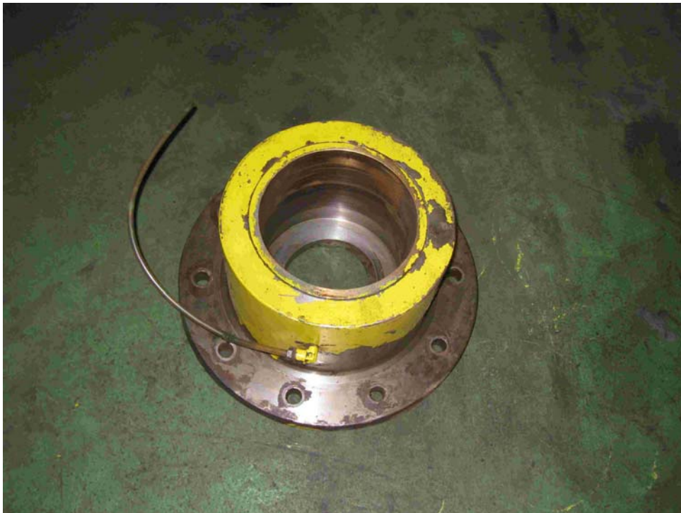
Fig.15: Lower Support Bush for the Arm and Hydraulic Support Frame of No.2 Dock Arm
