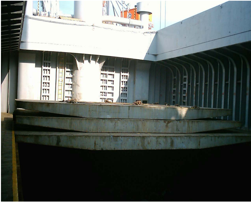
Fig 5 – The picture shows the stacked pontoons on tween deck of No. 2 cargo hold with the lifting sling wires for lifting by cargo crane
