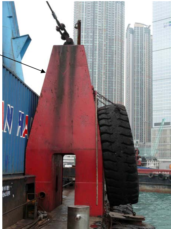
Fig. 2: Anchor Block of Slewing Guy on "Smart Hill No.1"
