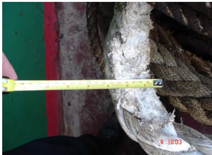
Fig. 6: Excessive wears at the eye of the other mooring rope.
