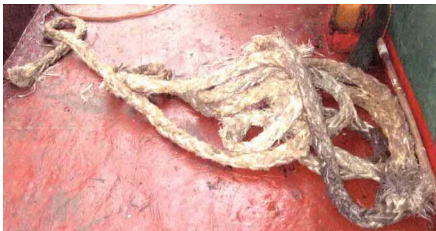
Fig. 4: The broken mooring rope
