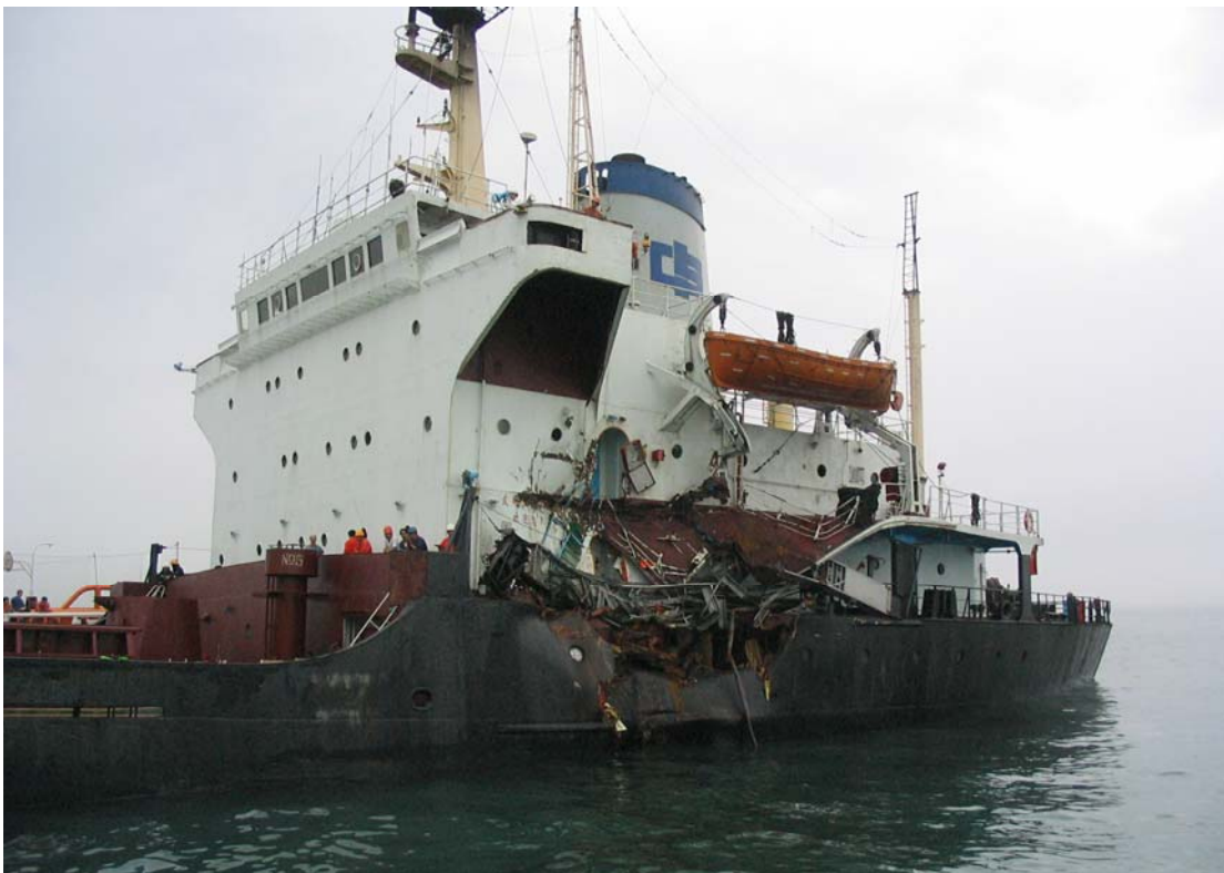
Figure 2 – Photograph showing the damages on port quarter of You Shun
