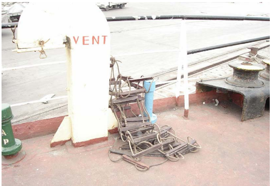
Figure 2 – Jacob Ladder secured on Handrail
