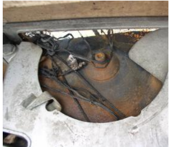
Fig. 7: Legwires were tangled at the circular saw cutter
