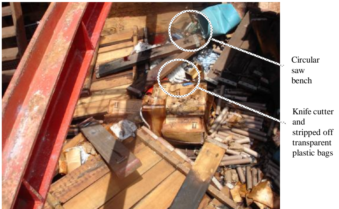
Fig. 5b: Condition of the cargo hold after the fire and the explosion
