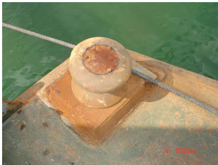
Fig. 1: A similar fairlead roller assembly
