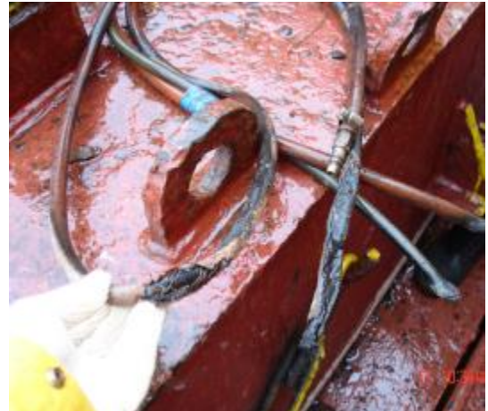
Fig.5: The burnt rubber hoses
