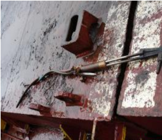
Fig.4: The gas-cutting torch
