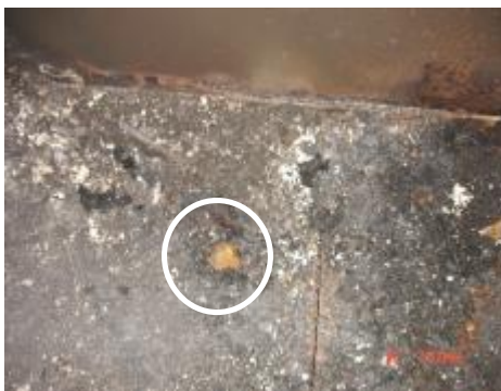
Fig. 13: Shoes of the Third Engineer was burnt, steel toecap remained on the floor.
