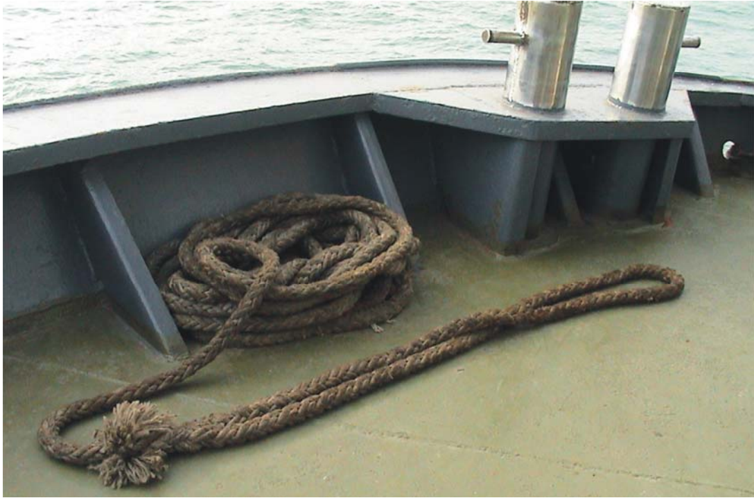
Figure 1 The height of the bulwark is about 235 mm
