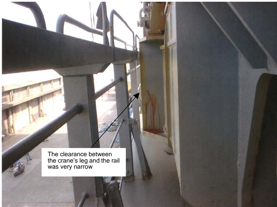
Figure 1 The clearance in between the crane leg to the ship's rail was narrow
