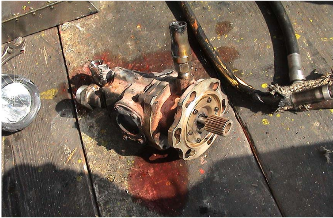
Fig. 1 : Engine starter with the seized splined drive coupling
