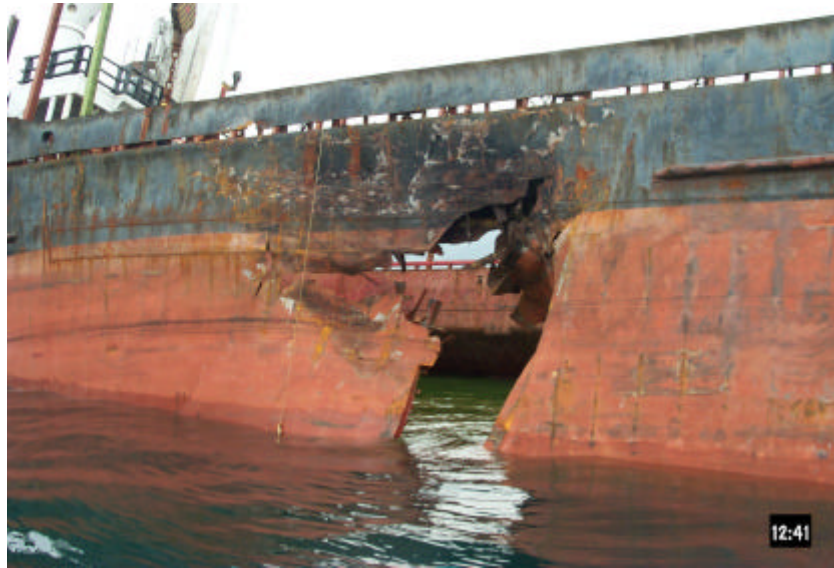
Fig. 1 Collision damage of “Ogrady”
