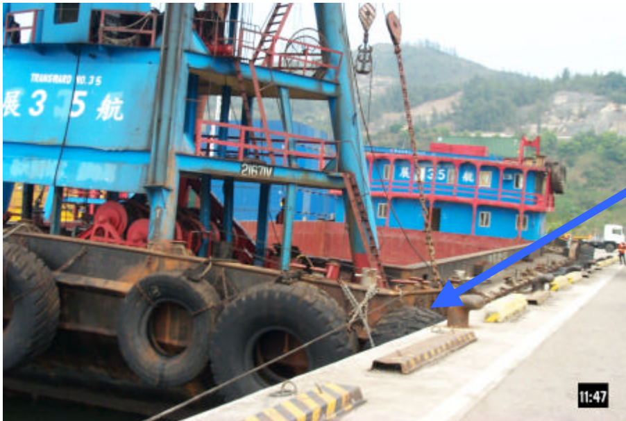
Fig. 1 A similar Lighter at moor in River Trade Terminal (Note the location of forward fender and the bollard)
