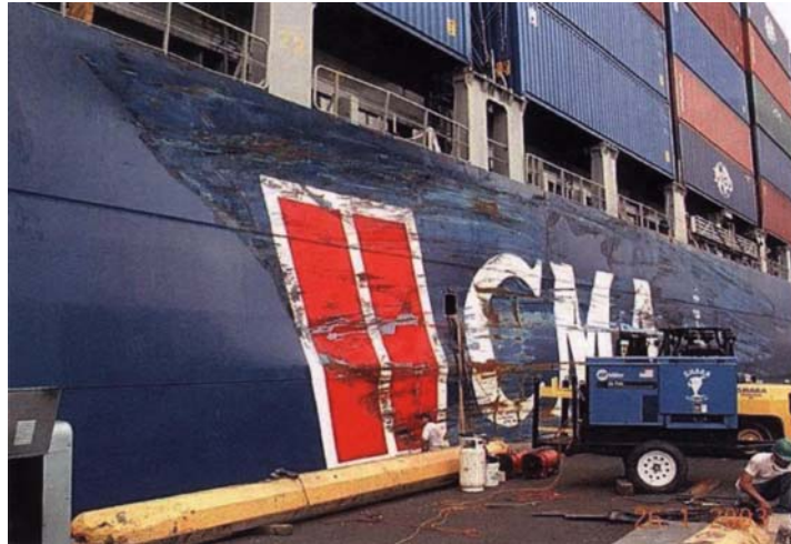
Figure 3 Collision damages of “Ville d’Orion”
