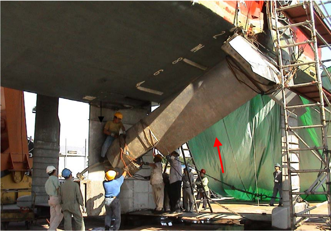
Fig. 1: Forward strut stuck between the aft struts
