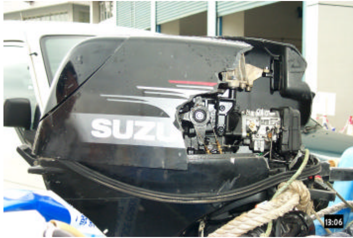
Fig. 3 Damages to the casing of the outboard engine
