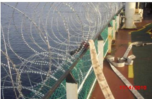
Fire Hoses rigged at various locations
